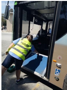
Putting down the ramp
